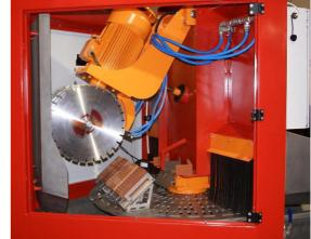
to the rear providing the collection of the big amounts of water and slurry into the water bin underneath the machine. This way of designing prevents the sensible components as motors and actuators from being polluted unnecessary.
